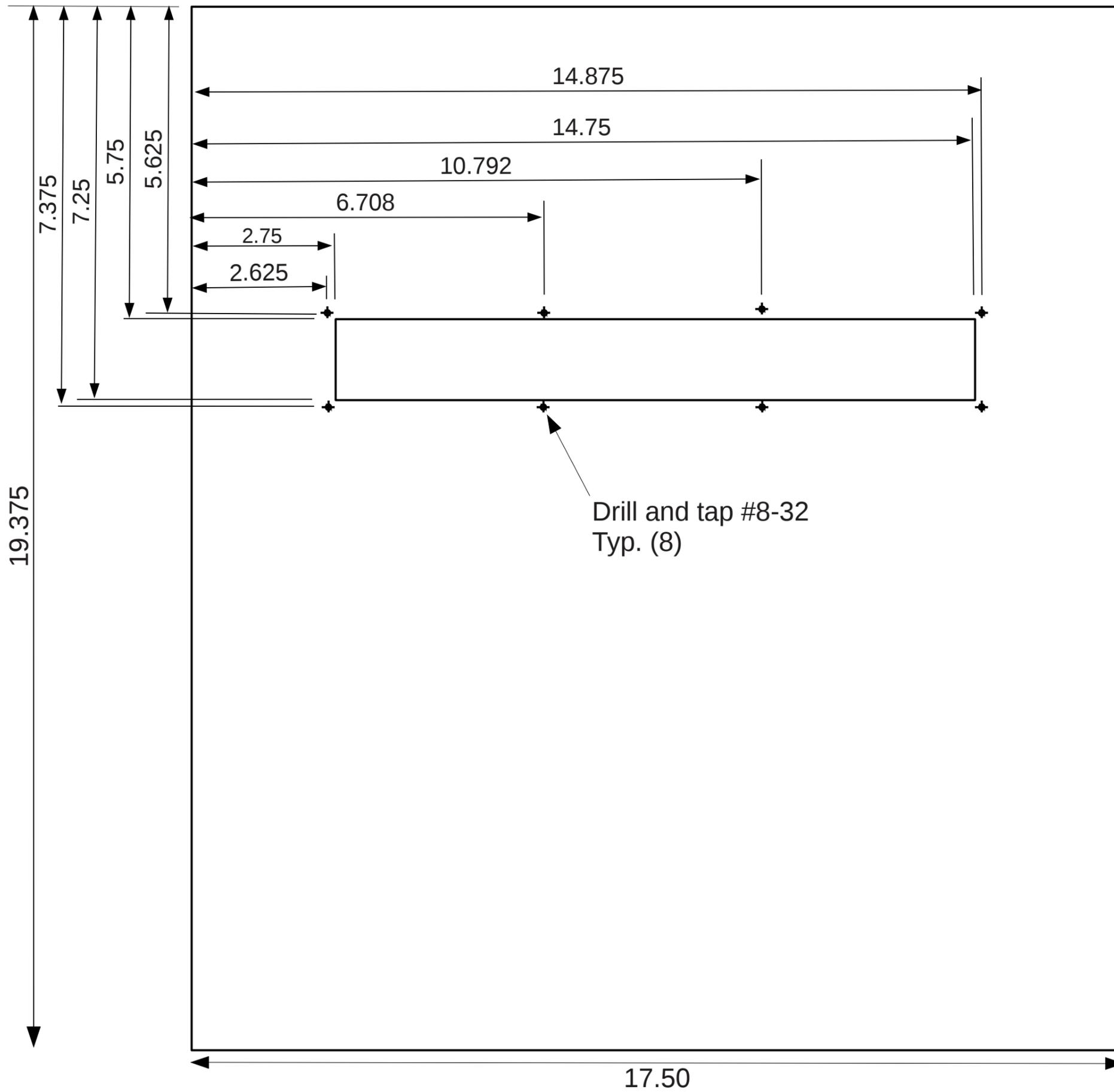
12" x 1.5" slot in existing equipment box panel
