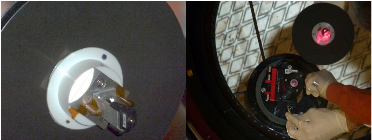
Figure 18: Left: The rail mounted handgun laser mounted to a delrin cap at the center of the ASM. The laser acts as an optical axis boresight reference and is also used to verify the location of the CRO. Right: The CRO cup mounted to its piezo stage and magnetic kinematic mount. The boresight laser is shining directly into the hole in the CRO return flat, indicating a good alignment. This view is the reflection in the ASM.
