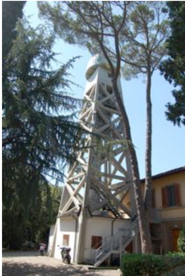
Figure 15: The ASM test setup in the Arcetri test tower. The concave secondary allows for a relatively simple double-pass optic test configuration at the same focal length that it will be used at the telescope. A calibration source in the NAS at the far focus reflects off of the ASM, then the CRO, then back to the CRO before entering the W-unit for wavefront sensing and technical viewing.
