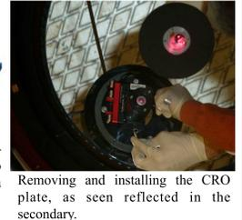
Removing and installing the CRO plate, as seen reflected in the secondary.
