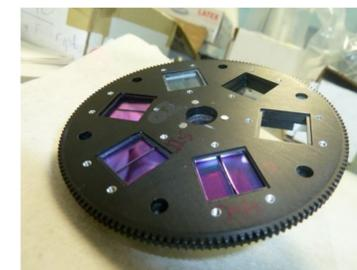
The coronagraph wheel with its prototype SDI filter pairs and coronagraphic spots.
