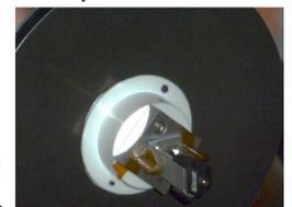
A removable handgun laser can be mounted on a delrin cap in the center of the ASM for use both to verify the CRO position and as a boresight reference.
