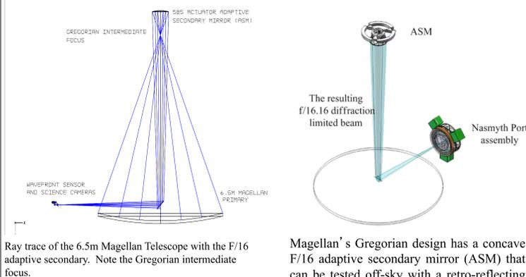
Ray trace of the 6.5m Magellan Telescope with the F/16 adaptive secondary. Note the Gregorian intermediate focus.
