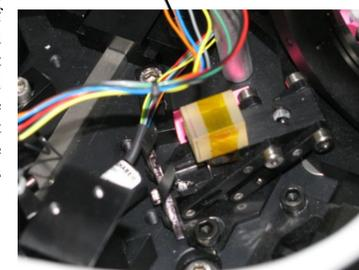
Our prototype quartz Wollaston prism mounted on its elevator stage that can be raised and lowered in and out of the beam. Ultimately we have adopted a calcite design. The larger birefringence of calcite allows for a much more shallow cut angle and thinner prism that minimizes astigmatism introduced into the beam.
