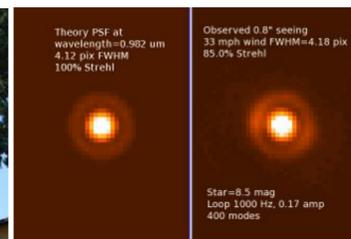
Closed loop performance at 982 nm of the complete AO system in the Arcetri test tower. (a) Theoretical PSF at this F/# and wavelength. (b) AO corrected image of the fiber source with the tower vibration, ambient environment, and injected "seeing" as the sources of turbulence.
