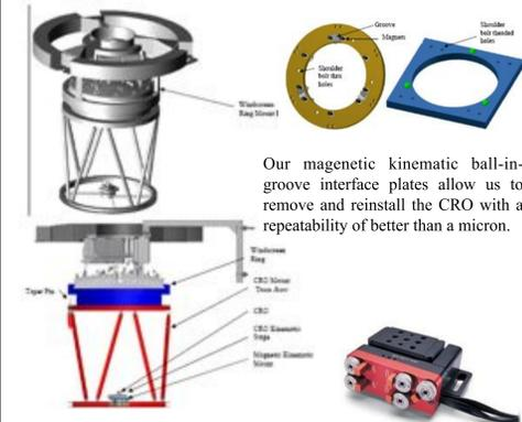
Our magnetic kinematic ball-in-groove interface plates allow us to remove and reinstall the CRO with a repeatability of better than a micron.
