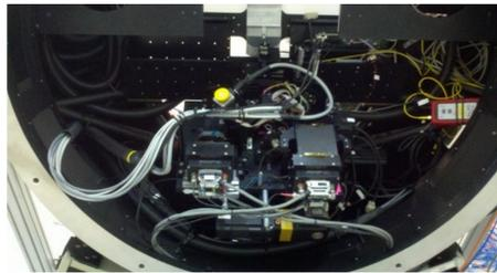
The W-Unit contains the pyramid wavefront sensor (WFS) and the VisAO science and acquisition camera.
