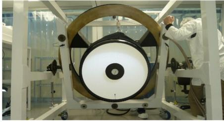
Our 585 element adaptive secondary mirror (ASM) in the cleanroom at LCO.
