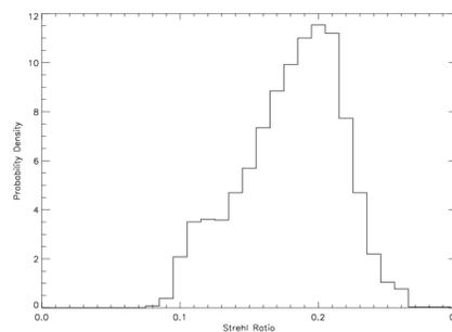
The probability density function and cumulative distribution of the short exposure Strehl. For this experiment the loop was intentionally degraded, operating at 500Hz on a 9th mag star with gain set somewhat high to be unstable. This was necessary to generate a time series with enough variability to test RTFS. Though a laboratory artificiality, simulations and prior work in closed loop AO show that the achieved SR distributions and variability are realistic for fainter stars.
