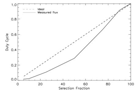
Duty cycle, measured photometrically, compared to the selection fraction. This plot is a good proxy for accuracy: a perfectly accurate system would follow the  $y=x$  line. The current implementation, with no prediction algorithms in use, tends to under select, resulting in a lower than expected duty cycle.
