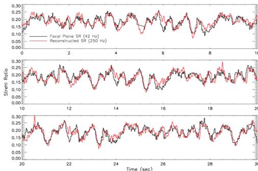
Measured short exposure (42fps) and reconstructed SR. The reconstructed SR is calibrated using the short exposure time series by matching the spread (std. dev.) and mean. The reconstructed SR is also low-pass filtered in real-time to suppress high frequencies which would over-drive the shutter.
