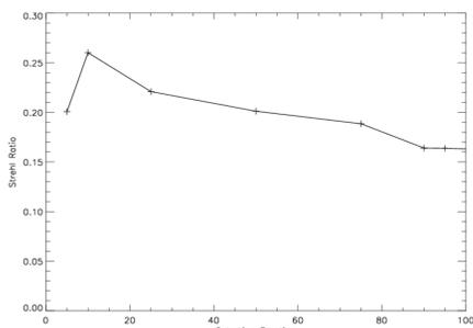
Long exposure SR vs. the selection threshold. A threshold of 50% implies that the system attempts to open the shutter whenever SR was above the median short exposure value. The shutter has a finite actuation time of about 10msec. The drop in achieved SR when only the best 5% was selected is likely due to this actuation delay compared to the narrowness of the corresponding SR peaks in the time series.
