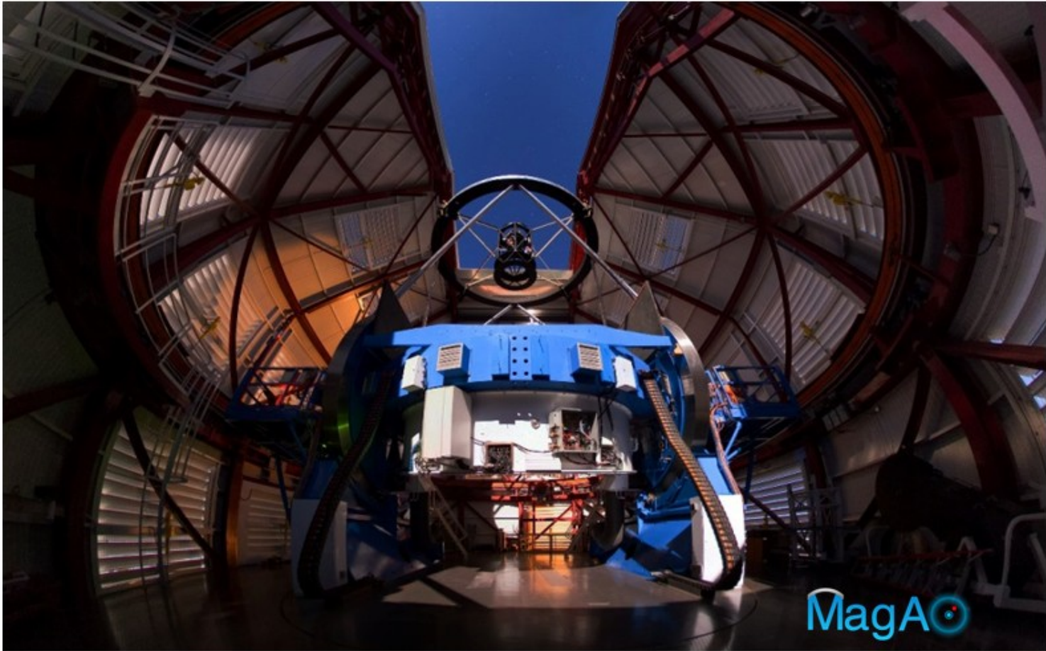
Figure 1: The Magellan Telescope with MagAO's Adaptive Secondary Mirror (ASM) mounted at the top looking down (some 9 meters) onto the 6.5m (21 foot) diameter Primary Mirror (not visible, inside blue mirror cell). Moonlight image, credit: Yuri Beletsky, Las Campanas Observatory.
