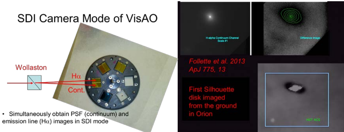
Fig 7: A cartoon of the SDI mode (left). To the right we see a real science example of the SDI mode in action. Here we see how a young forming solar system has its dust traced out by the shadow it casts as the bright Halpha background is absorbed by its dust disk. Modified from Follette et al. 2013.
