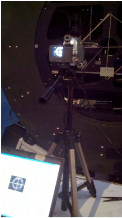
Figure 4. Alignment of MagAO. At right is a diagram of the optical path, including the intermediate focus located just below the ASM (base diagram from http://www.lco.cl/telescopes-information/magellan/ , see Shectman 1994 23 for more on the Magellan Clay optical design). At center is a photo of the W-unit mounted on the NAS, without Clio2 so that there is a clear sight to the ASM from the NAS platform. At left is a photo of the video camera set-up to align the ASM with the telescope optical axis. The NAS ring with a string cross-hair is clearly seen at the center of both photos.
